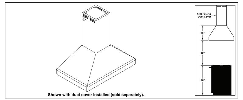
3) Load-bearing framework in the ceiling is necessary for the installation of an island hood. Additional framework construction may be required. Do not attach an island hood to a structure that cannot support twice the weight of the hood.
