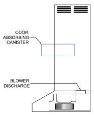
13) Move the canister all the way to the back and then lower the canister over the blower discharge. Shift the canister front to back and left to right to make sure that the blower discharge and canister have fully engaged.
