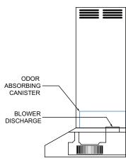
14) With the gasket side facing down, nest the smoke trapping filter element into the pocket that forms the top of the odor absorbing canister. The filter may have a rectangular base so rotate as necessary. Replace the duct cover front panel by aligning the snaps and pressing each snap into position.
