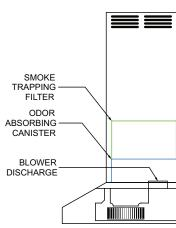
15) Refer to the Owner Maintenance Guide for Models Equipped with K250 Blower for proper hood operation. Test all blower and light functions to ensure they are operating properly.
