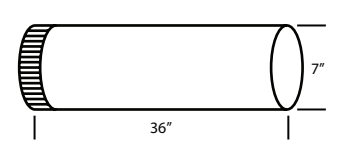
ROUND DUCT PIPE
