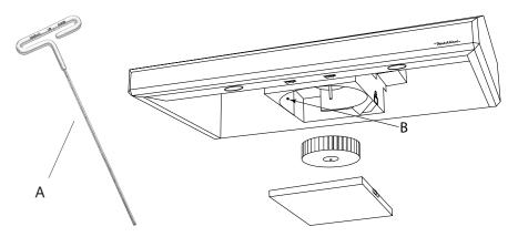
A soft bristle toothbrush with warm soapy water may be used to clean the blades, or soak the blower wheel in warm soapy water. When reinstalling the wheel onto the motor shaft, make sure the set screw makes direct contact with the "flat spot" on the motor shaft. Slide the blower wheel onto the motor shaft as far as it will go and tighten the set screw (clockwise) to lock the blower wheel in the correct position.
