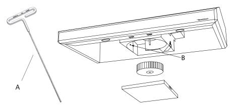
A soft bristle toothbrush with warm soapy water may be used to clean the blades, or soak the blower wheel in warm soapy water. When reinstalling the wheel onto the motor shaft, make sure the set screw makes direct contact with the "flat spot" on the motor shaft. Slide the blower wheel onto the motor shaft as far as it will go and tighten the set screw (clockwise) to lock the blower wheel in the correct position.
