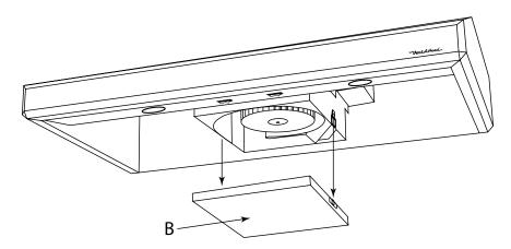
Clean the grease pan in a sink of warm, soapy water (liquid dish detergent) and let soak for a few minutes. Wash with a sponge or dishcloth, rinse and let drain. Reinstall the grease pan and snap the suitcase latches in place. The grease pan alternatively may be placed into a dishwasher.
